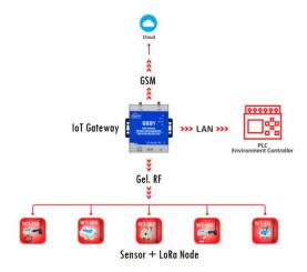
Fig. 2. IoT gateway diagram block.
