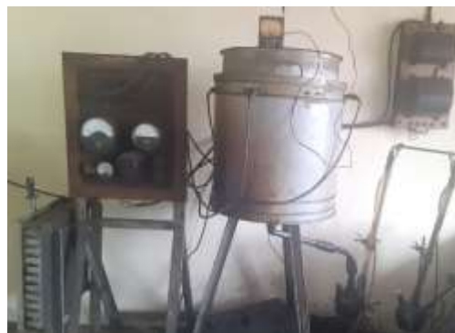
Figure 1. Electric retort for carbonization process
