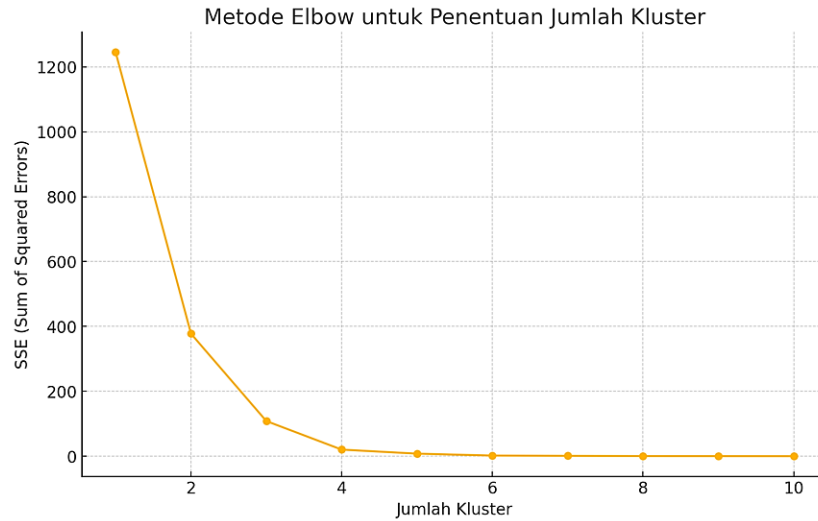
Fig. 2. Elbow Method to Determine Number of Cluster
