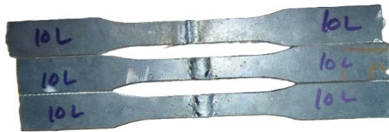
Fig 2. Tensile test specimens used for 10 liters/minute variable.
