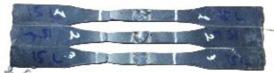
Fig 3. Tensile test specimens used for 15 liters/minute variable.
