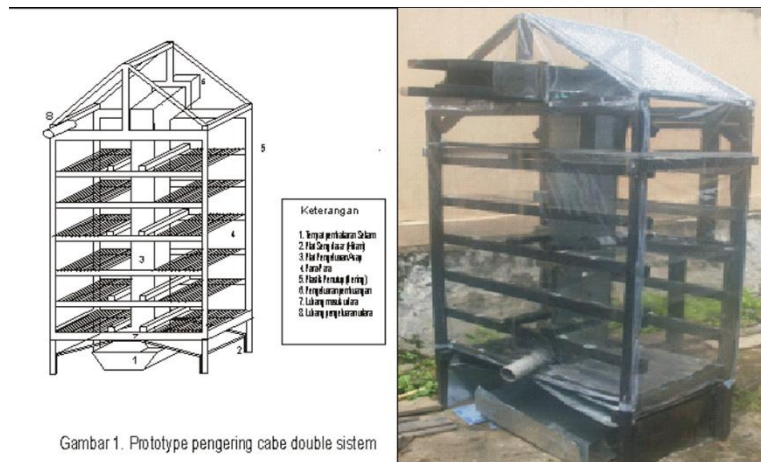
Gambar 5. Hasil rancangan alat pengering model hybrid Sumber: Yamin et al. (2023)
